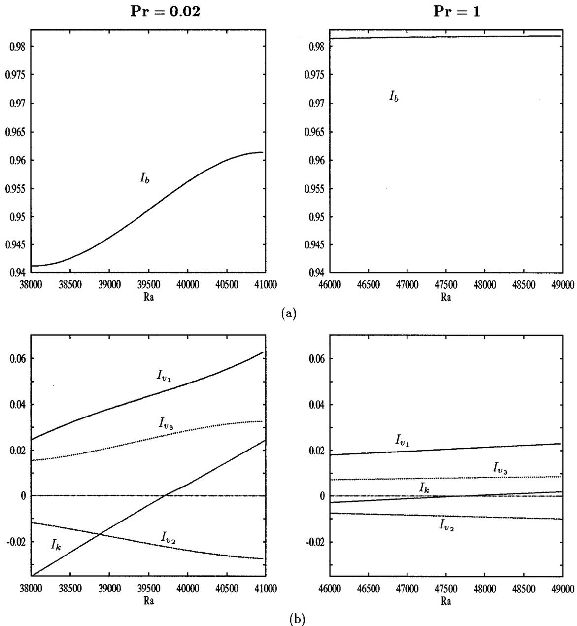
FIG. 8. Main kinetic energy contributions for  $Pr=0.02$  and  $Pr=1$ , around the secondary bifurcation point. Evolution of the buoyancy term  $I_b$  (a), the rate of change of kinetic energy  $I_k$ , and the main kinetic energy production terms  $I_{v_1}$ ,  $I_{v_2}$ , and  $I_{v_3}$  (b) as a function of  $Ra$  ( $A=0.5$ ).
