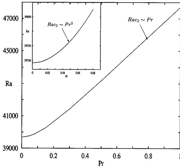
FIG. 7. Influence of the Prandtl number on the secondary bifurcation (from  $m=0$  to  $m=02$ ) for  $A=0.5$ . Evolution of the secondary threshold  $Ra_{c2}$  as a function of  $Pr$ .
