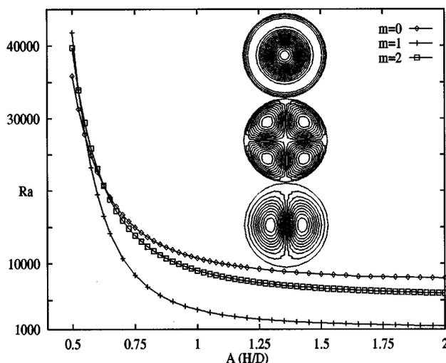
FIG. 4. Influence of the aspect ratio on the onset of convection. Evolution of the primary thresholds  $Ra_c$ , corresponding to the modes  $m=0$ ,  $m=1$ , and  $m=2$ , as a function of  $A$ .
