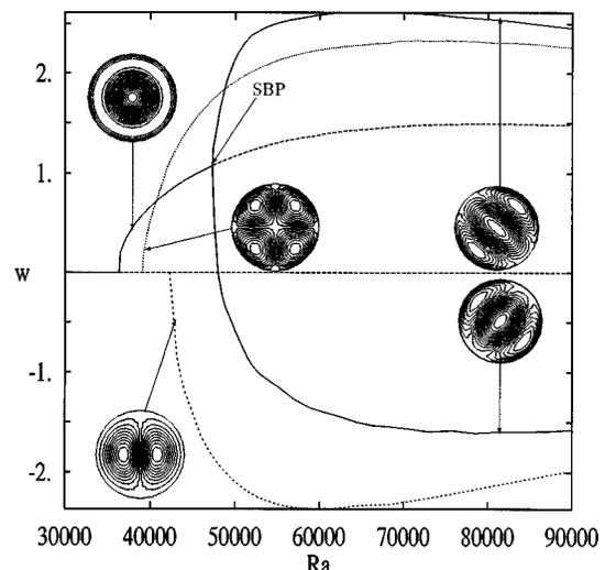
FIG. 6. Bifurcation diagram giving the evolution of the vertical velocity  $w$  at a fixed point as a function of the Rayleigh number,  $Ra$ . Plots of contours of  $w$  in the horizontal midplane. SBP: secondary bifurcation point ( $A=0.5$  and  $Pr=1$ ).
