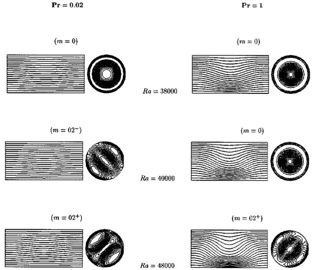
FIG. 12. Evolution of the convective structure of the steady stable solution for Pr=1 and Pr=0.02. Isotherms in the vertical symmetry plane and contours of the vertical velocity in the midplane  $P_H$ , before and after the secondary bifurcation from the mode  $m=0$  to the mode  $m=02$  (A=0.5).
