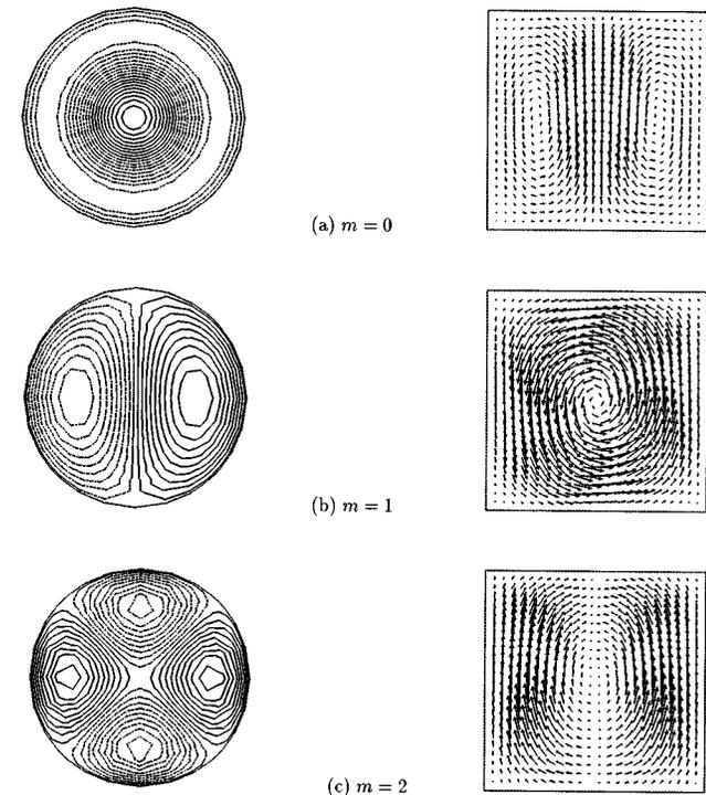
FIG. 3. The three principal modes, (a)  $m=0$ , (b)  $m=1$ , and (c)  $m=2$ . Left-hand side: contours of the vertical velocity  $w$  in the horizontal plane  $P_H$ . Right-hand side: velocity field in a vertical midplane ( $A=1$ ).
