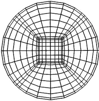
FIG. 2. Space discretization: the cavity is divided into five macro-elements (use of the isoparametric spectral element method).
