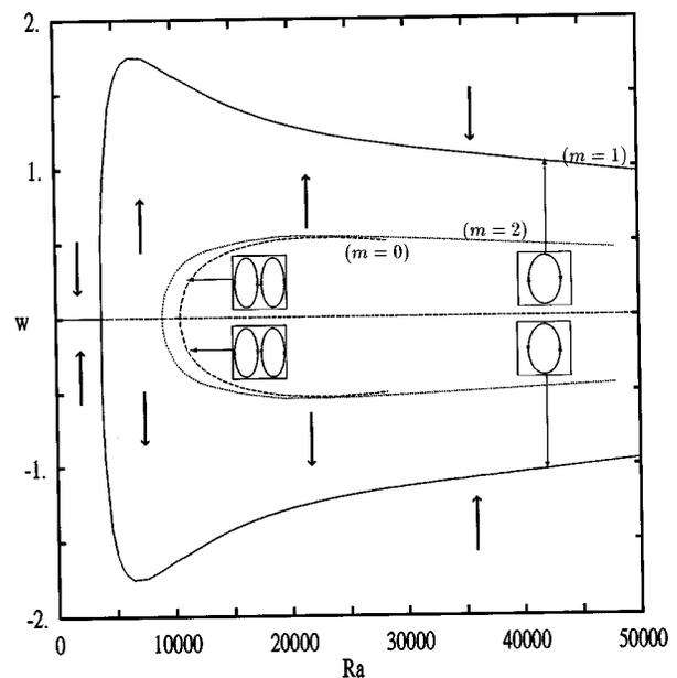
FIG. 5. Bifurcation diagram giving the evolution of the vertical velocity  $w$  at a fixed point as a function of the Rayleigh number,  $Ra$  ( $A=1$  and  $Pr=1$ ).
