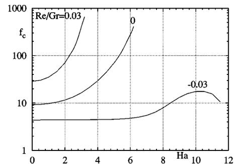
FIG. 8. Variation of the critical frequency  $f_c$  as a function of  $Ha$  for three values of  $Re/Gr$  ( $Pr=0.02$ ).
