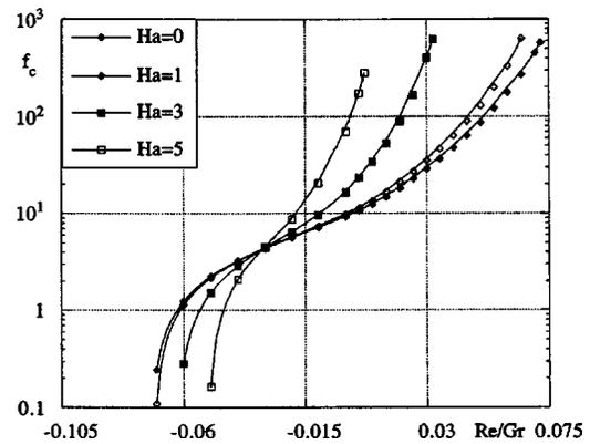
FIG. 7. Variation of the critical frequency  $f_c$  as a function of  $Re/Gr$  for different values of  $Ha$  ( $Pr=0.02$ ).
