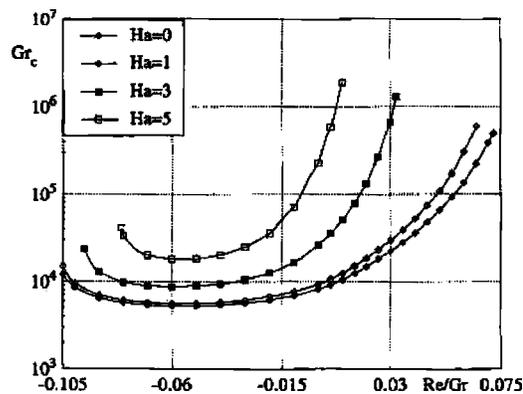
FIG. 3. Variation of the thresholds  $\text{Gr}_c$  as a function of  $\text{Re}/\text{Gr}$  for different values of  $\text{Ha}$  ( $\text{Pr} = 0.02$ ).
