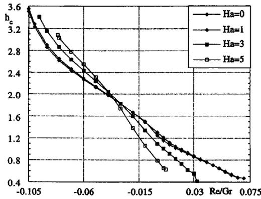
FIG. 5. Variation of the critical wavenumbers  $h_c$  as a function of  $Re/Gr$  for different values of  $Ha$  ( $Pr=0.02$ ).
