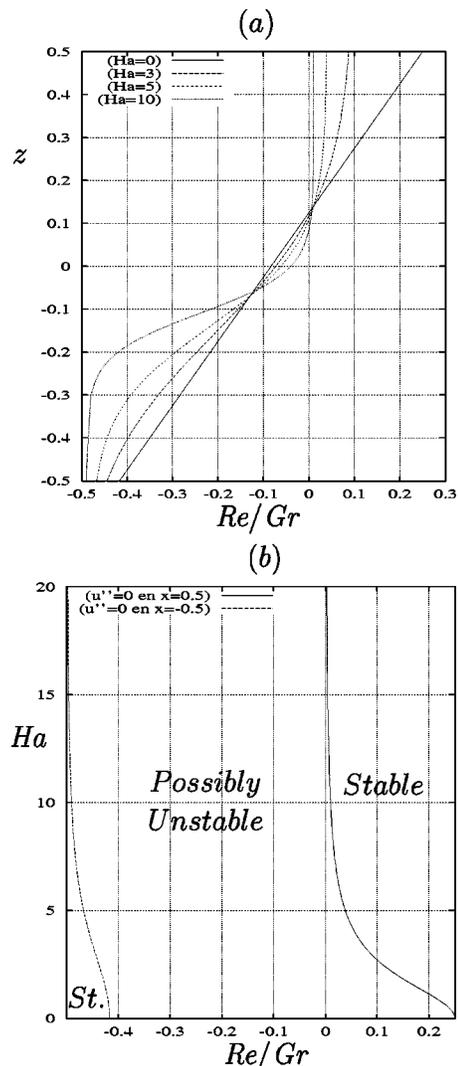
FIG. 9. (a) Variation of the position of the inflexion point in the velocity profiles when  $Re/Gr$  is changed for different values of Ha; (b) limits of the profiles with an inflexion point in terms of  $Re/Gr$  as a function of Ha, indicating limits of stability in the frame of the inviscid theory.
