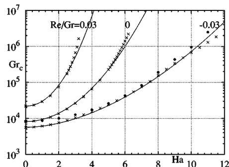
FIG. 4. Variation of the thresholds  $\text{Gr}_c$  as a function of  $\text{Ha}$  for three values of  $\text{Re}/\text{Gr}$  ( $\text{Pr} = 0.02$ ). The symbols (X) correspond to the calculated results and the lines to well-correlated characteristic laws given in the text. For comparison, the symbols (•) indicate the results for the rigid situation.
