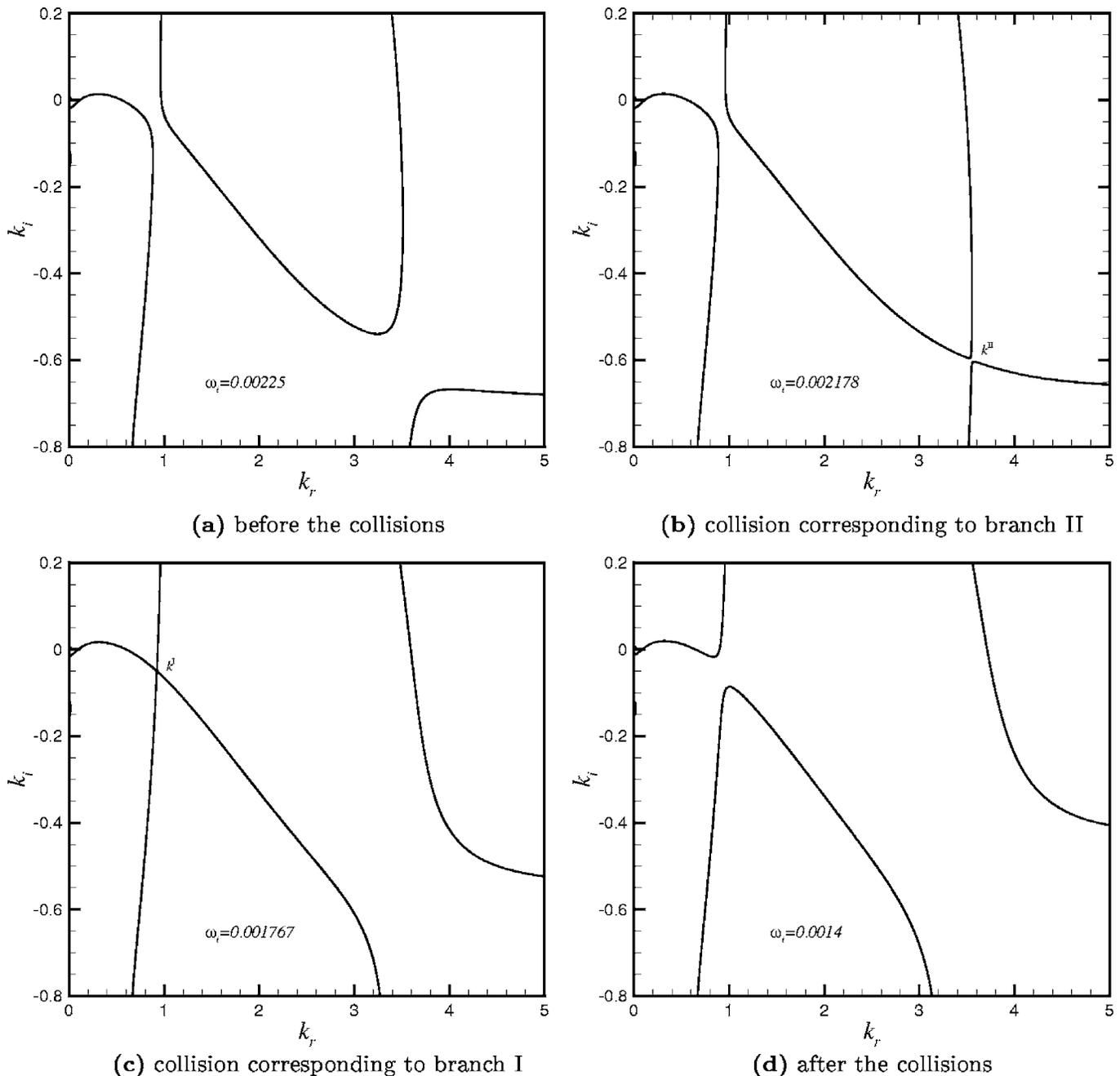
FIG. 8. Pinching process in the complex wave number plane  $(k_r, k_i)$  for  $V=1.2195$ ,  $m=2.5$ ,  $\gamma=1$ ,  $\delta=1$ , and  $\theta=0.2$ .
