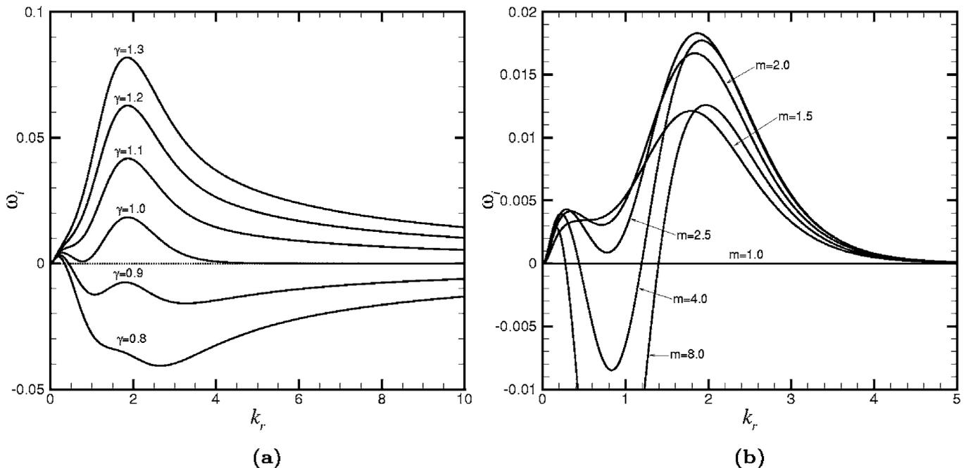
FIG. 3. Growth rates of the inertialess interfacial instability for (a)  $m=2.5$  and different density ratios  $\gamma$ , and (b)  $\gamma=1.0$  and different viscous ratios  $m$  ( $\delta=1$  and  $\theta=0.2$ ).
