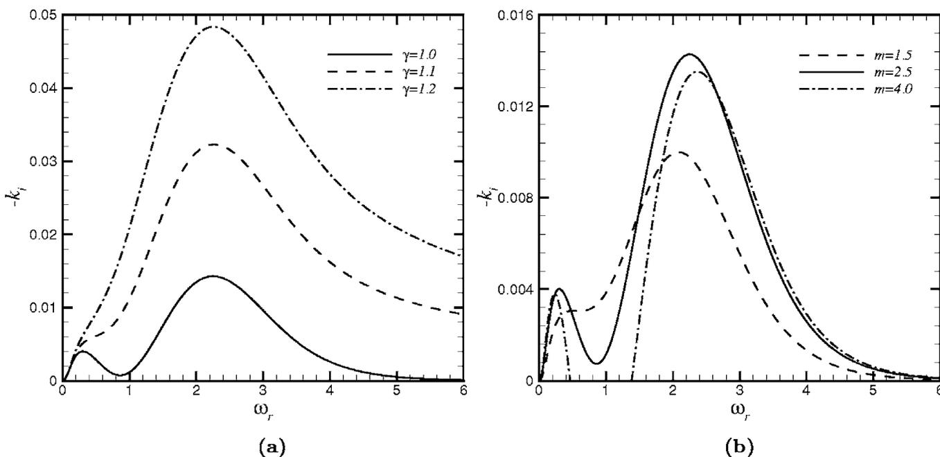
FIG. 12. Spatial growth rate  $-k_i$  as a function of the forcing frequency  $\omega_r$  for (a)  $m=2.5$  and different density ratios, and (b)  $\gamma=1.0$  and different viscous ratios ( $\delta=1$  and  $\theta=0.2$ ).
