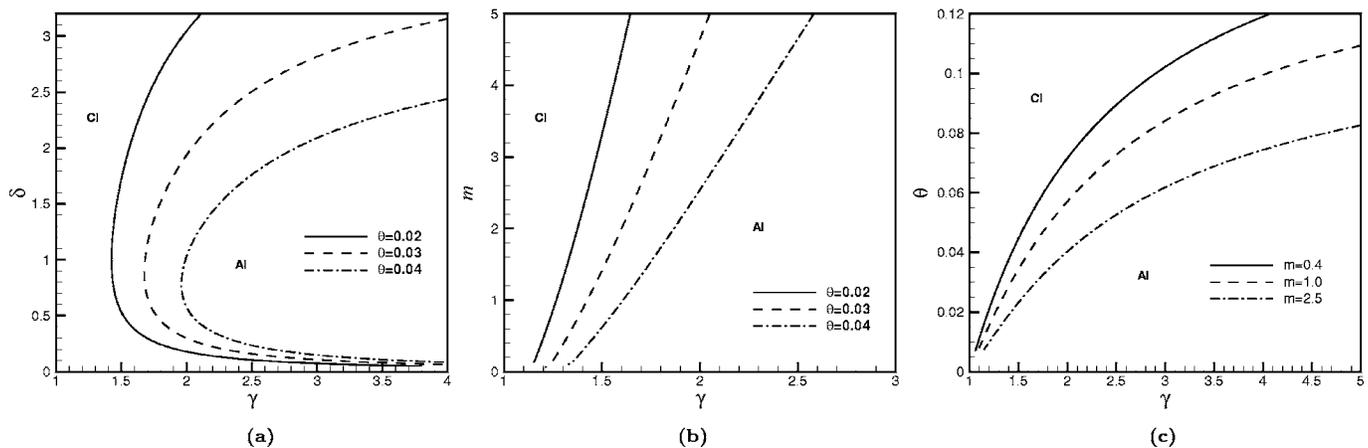
FIG. 11. Boundary curves between absolute and convective instability: (a)  $\delta-\gamma$  curves for  $m=2.5$  and different incline angles, (b)  $m-\gamma$  curves for  $\delta=1.0$  and different incline angles, and (c)  $\theta-\gamma$  curves for  $\delta=1.0$  and different viscosity ratios.
