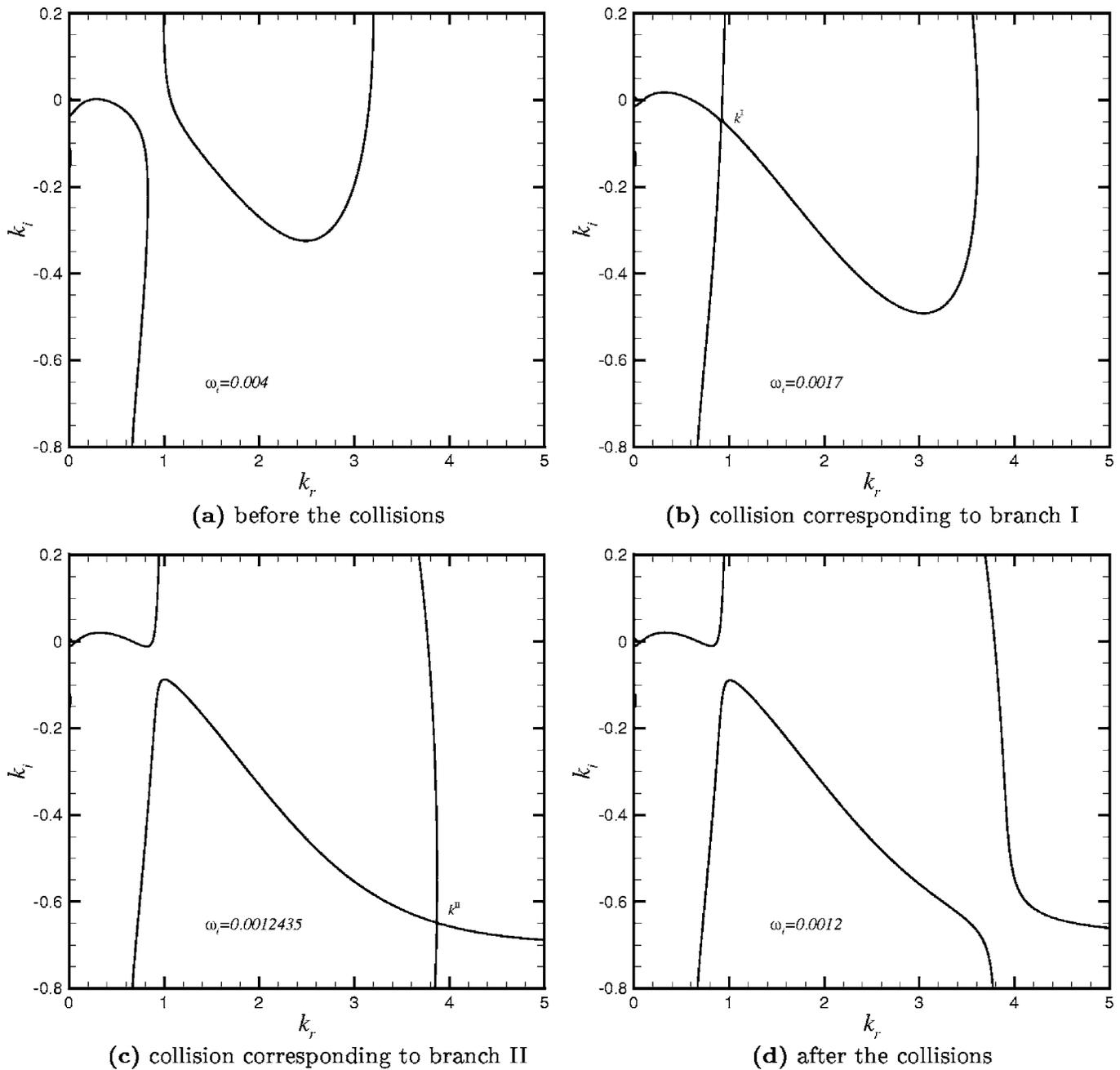
FIG. 9. Pinching process in the complex wave number plane  $(k_r, k_i)$  for  $V=1.218$ ,  $m=2.5$ ,  $\gamma=1$ ,  $\delta=1$ , and  $\theta=0.2$ .
