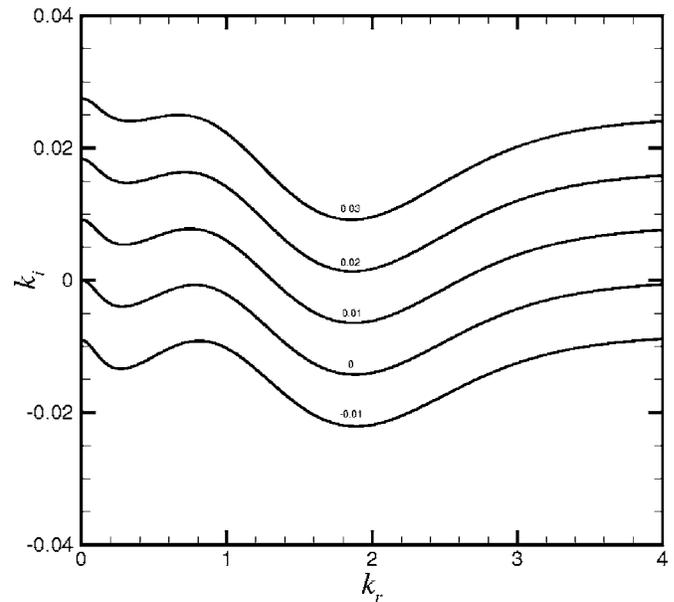
FIG. 5. Deformation of the spatial branches  $k_n(\omega)$  for decreasing growth rates  $\omega_i$  from 0.03 to  $-0.01$  for the case  $m=2.5$ ,  $\gamma=1$ ,  $\delta=1$  and  $\theta=0.2$ .
