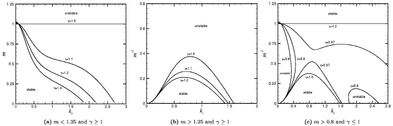
FIG. 2. Neutral curves of the inertialess interfacial instability for different density ratios  $\gamma$  in the  $m-k$  parameter space for  $\delta=1.0$  and  $\theta=0.2$ .
