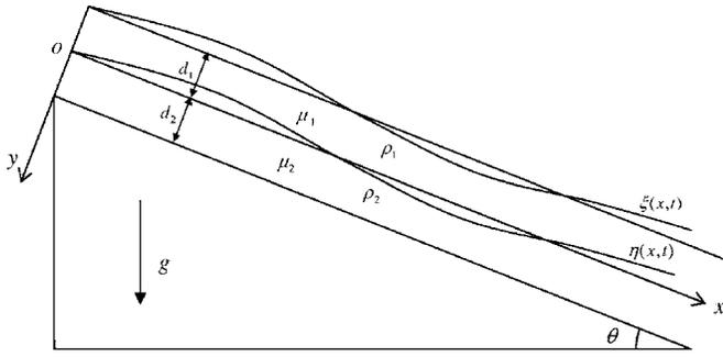
FIG. 1. Sketch map of the two layer film flow along an inclined plate.
