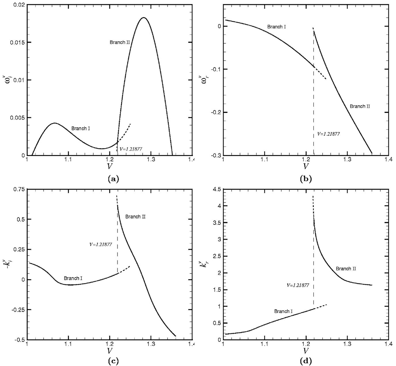
FIG. 7. (a) Growth rate  $\omega_i^v$ , (b) oscillatory frequency  $\omega_r^v$ , (c) local spatial amplification rate  $-k_i^v$ , and (d) local spatial wave number  $k_r^v$  as a function of the ray velocity  $V$ , for  $m=2.5$ ,  $\gamma=1$ ,  $\delta=1$ , and  $\theta=0.2$ .
