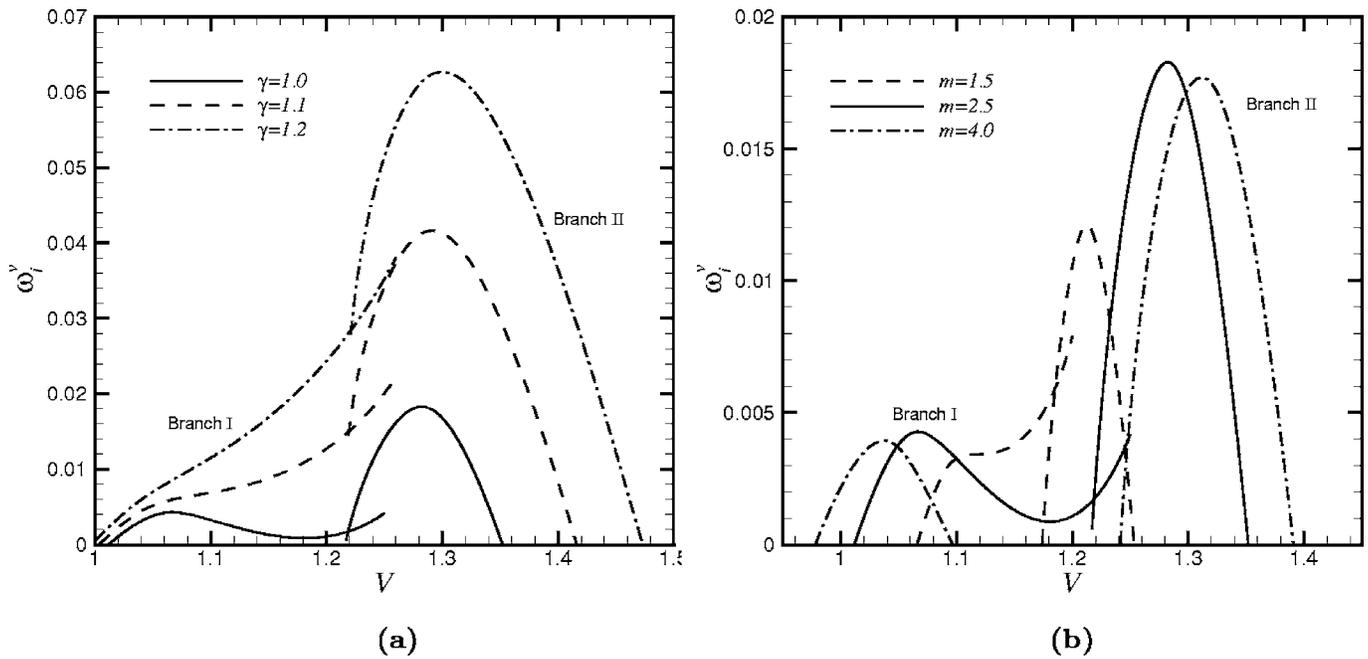
FIG. 10. Growth rate  $\omega_i^v$  as a function of the ray velocity  $V$  for (a)  $m=2.5$  and different density ratios, and (b)  $\gamma=1.0$  and different viscous ratios ( $\delta=1$  and  $\theta=0.2$ ).
