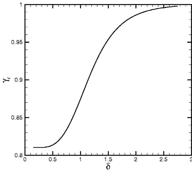
FIG. 4. Critical density ratios given as a function of the depth ratio and indicating the limit below which there does not exist finite wavelength interfacial instability for any large viscous ratio. The incline angle is  $\theta=0.2$ .
