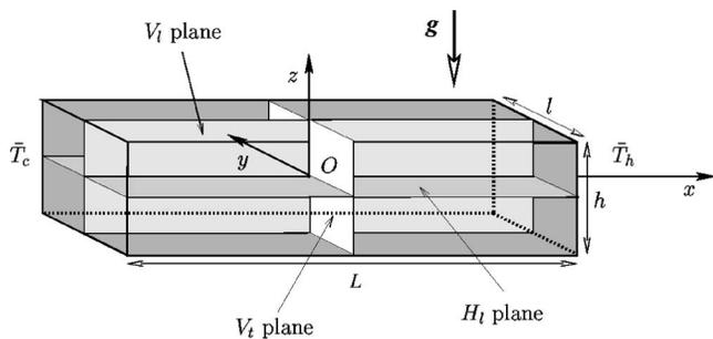
FIG. 1. Geometry of the differentially heated cavity.
