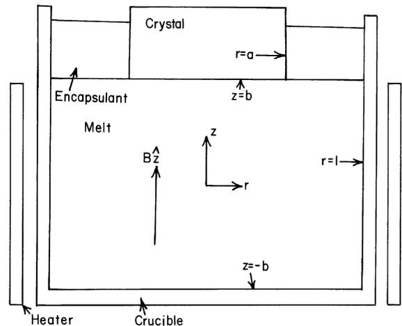
Fig. 1. Geometry with  $r$  and  $z$  normalized by the inside radius of the crucible and with the magnetic field  $B\hat{\mathbf{z}}$ .
