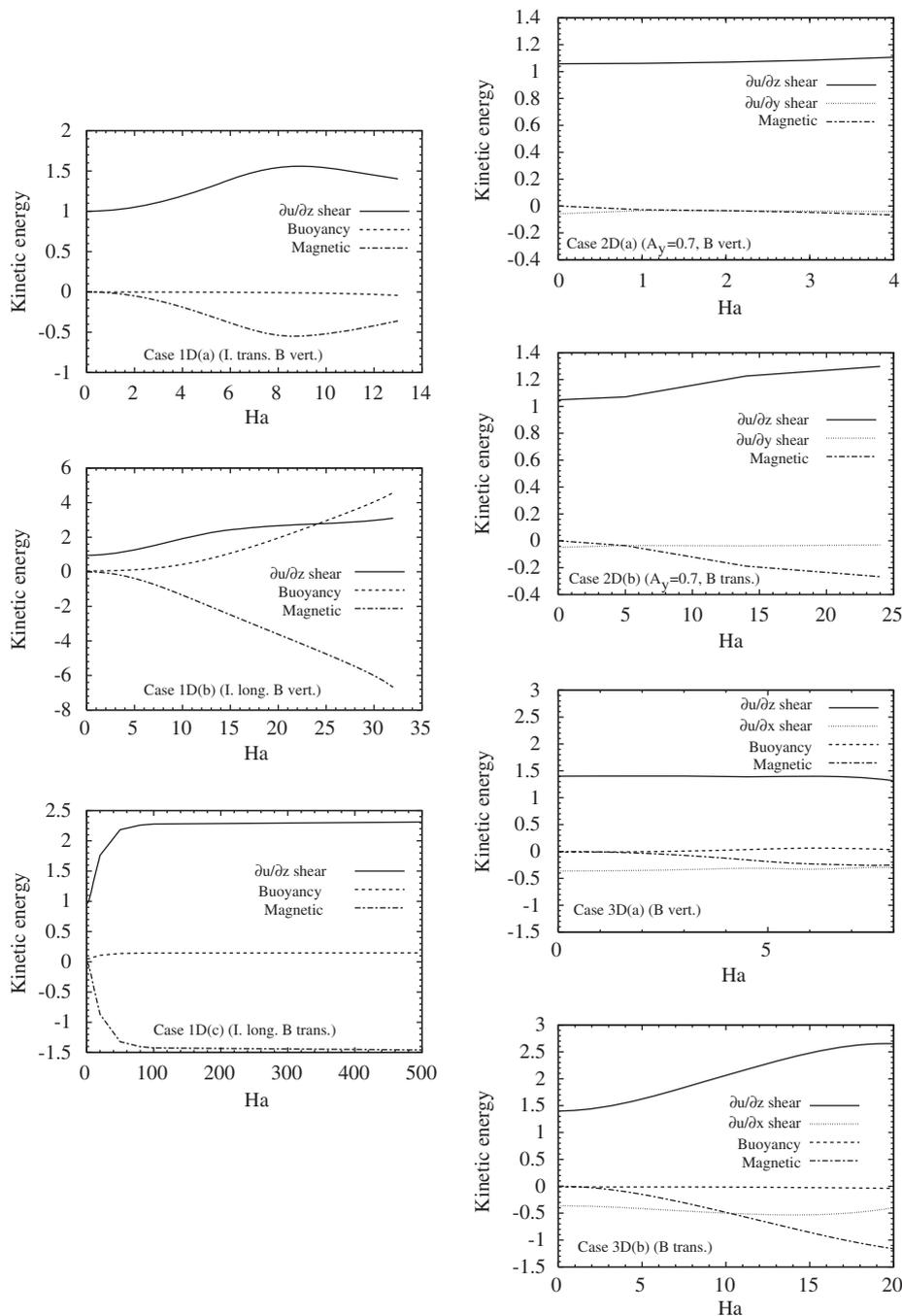
Fig. 4. Main contributions to the fluctuating energy budget (Eq. (7)) in the extended layer (cases 1D(a), 1D(b), 1D(c)), in the confined layer (cases 2D(a), 2D(b)) and in the 3D cavity (cases 3D(a), 3D(b)).
