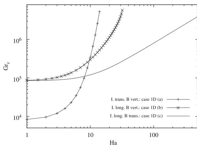
Fig. 1. Variation of the thresholds in the extended layer. In each case, the critical Grashof number  $Gr_c$  for the onset of instabilities is given as a function of the Hartmann number  $Ha$ .
