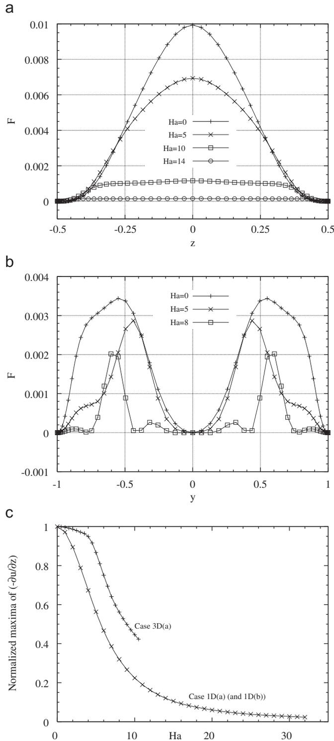
Fig. 5. Variation of the fluctuation part  $F$  of the dominant destabilizing shear energy  $S_{xz}$ : (a) in the case 1D(a) of the extended layer; (b) in the case 3D(a) of the 3D cavity. (c) Normalized variation of the maxima of  $-\partial u/\partial z$  at constant  $Gr$  for both cases.
