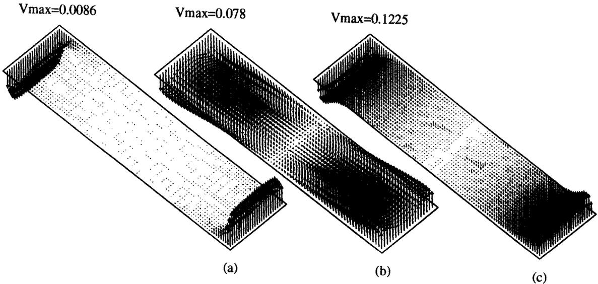
Fig. 7. Velocity vectors in the (Lh)-plane at  $Gr = 5 \times 10^4$  and  $Ha = 150$  for three orientations of the applied magnetic field ((a)  $B_y$  case, (b)  $B_z$  case, and (c)  $B_x$  case).
