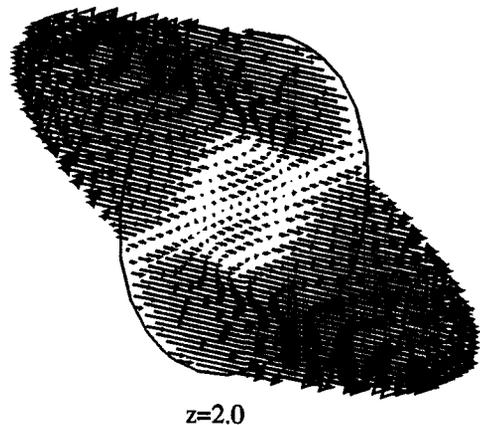
Fig. 11. Velocity vectors in the  $(Tv)$ -plane at  $Gr = 5 \times 10^4$  and  $Ha = 250$  in the  $B_z$  case.
