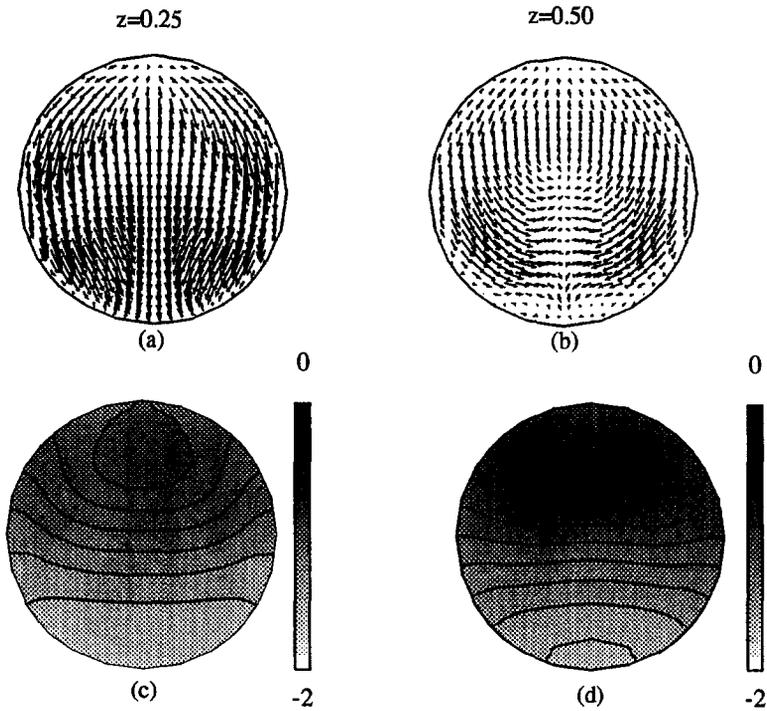
Fig. 4. Velocity vectors projection (a,b) and temperature isovalues (c,d) in cross-sectional planes at  $z = 0.25$  and  $z = 0.5$  for  $Gr = 1.5 \times 10^5$ ,  $Pr = 0.026$  and  $Ha = 0$ .
