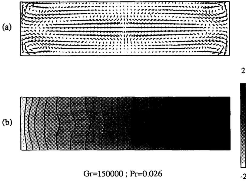
Fig. 3. Velocity vectors projection (a) and temperature isovalues (b) in the (Lh)-plane for  $Gr = 1.5 \times 10^5$ ,  $Pr = 0.026$  and  $Ha = 0$ .
