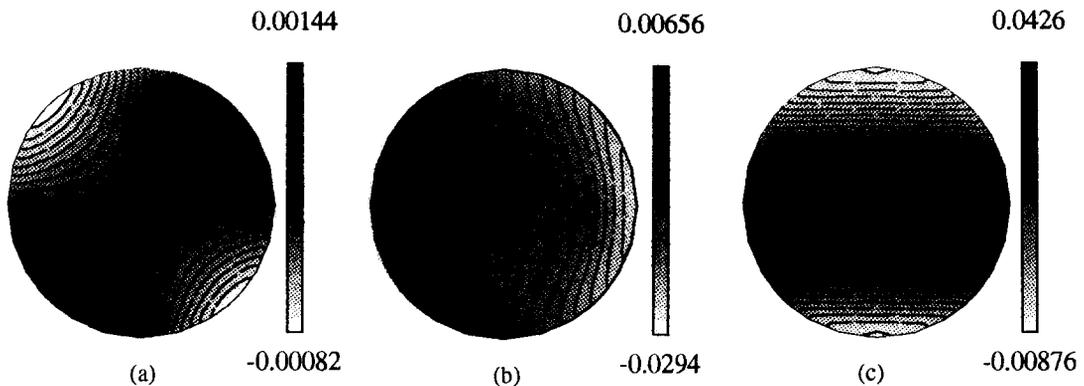
Fig. 9. The electric potential field in a cross-sectional plane ( $z = 0.5$ ) at  $Gr = 5 \times 10^4$  and  $Ha = 150$  for three orientations of the applied magnetic field ((a)  $B_y$  case, (b)  $B_z$  case and (c)  $B_x$  case) (view from the right).
