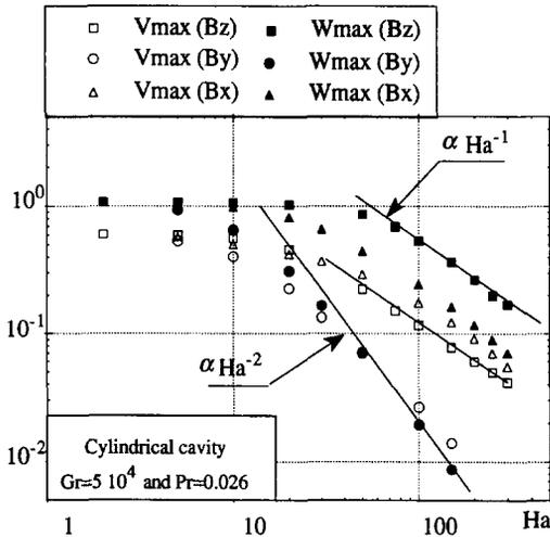
Fig. 10. Plots of the maxima of  $v$  and  $w$  as a function of  $Ha$  at  $Gr = 5 \times 10^4$  and  $Pr = 0.026$  for three orientations of the magnetic field.
