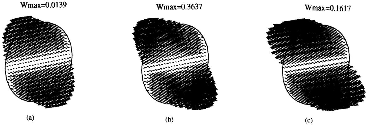
Fig. 6. Velocity vectors in the (Tv)-plane at  $Gr = 5 \times 10^4$  and  $Ha = 150$  for three orientations of the applied magnetic field ((a)  $B_y$  case, (b)  $B_z$  case, and (c)  $B_x$  case).
