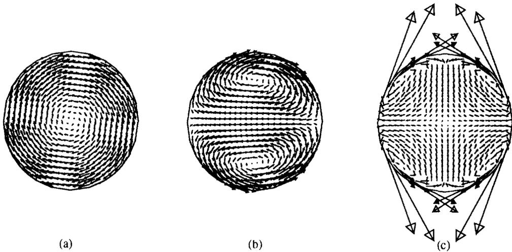
Fig. 8. The electric current projection in a cross-sectional plane ( $z = 0.5$ ) at  $Gr = 5 \times 10^4$  and  $Ha = 150$  for three orientations of the applied magnetic field ((a)  $B_y$  case, (b)  $B_z$  case, and (c)  $B_x$  case) (view from the right).
