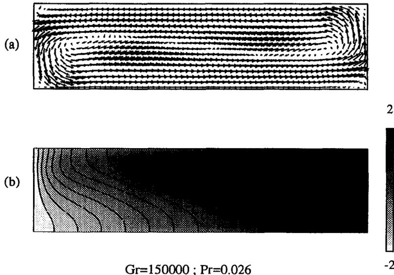
Fig. 2. Velocity vectors (a) and temperature isovalues (b) in the (Lv)-plane for  $Gr = 1.5 \times 10^5$ ,  $Pr = 0.026$  and  $Ha = 0$ .
