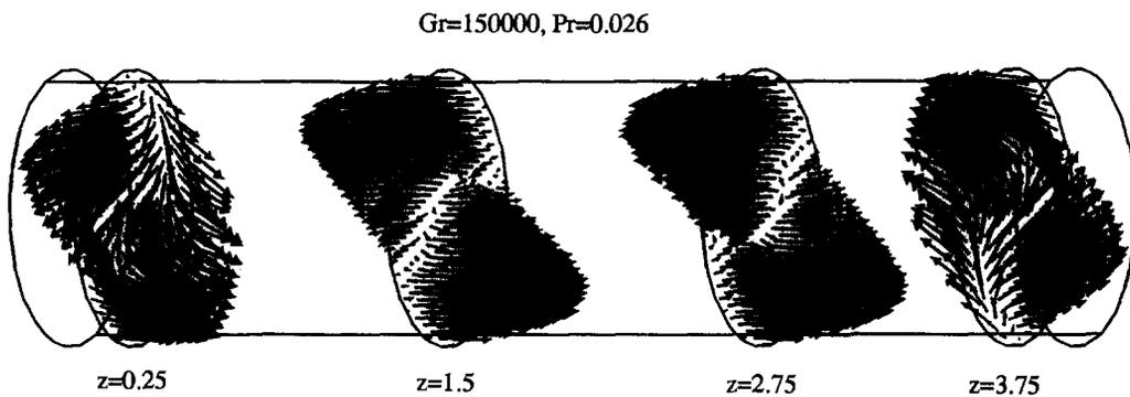
Fig. 5. Three-dimensional velocity vectors field given in four cross-sectional planes ( $z = 0.25, 1.5, 2.75, 3.75$ ) for  $Gr = 1.5 \times 10^5$ ,  $Pr = 0.026$  and  $Ha = 0$ .
