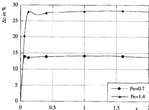
Fig. 5. Variation of the radial segregation  $\Delta c$  for  $Gr = 5000, k = 0.087, \Delta \xi = 6\%$  and different values of  $Pe$ .
