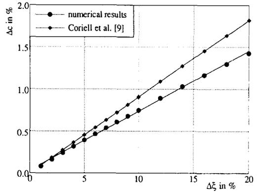
Fig. 2. Variation of the radial segregation  $\Delta c$  for the pure diffusive state.
