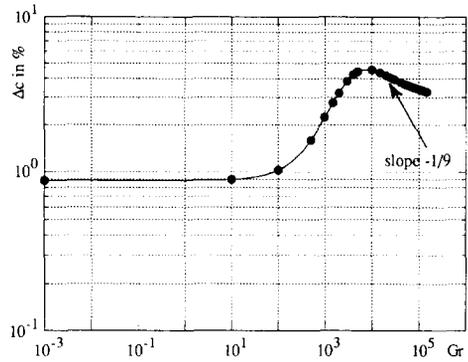
Fig. 6. Variation of the radial segregation  $\Delta c$  as a function of  $Gr$ .
