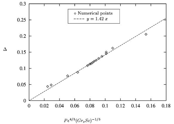
Fig. 8. Variation of  $\Delta$  as a function of  $Pe$ ,  $Gr_s$  and  $Sc$  under the analytical model law.
