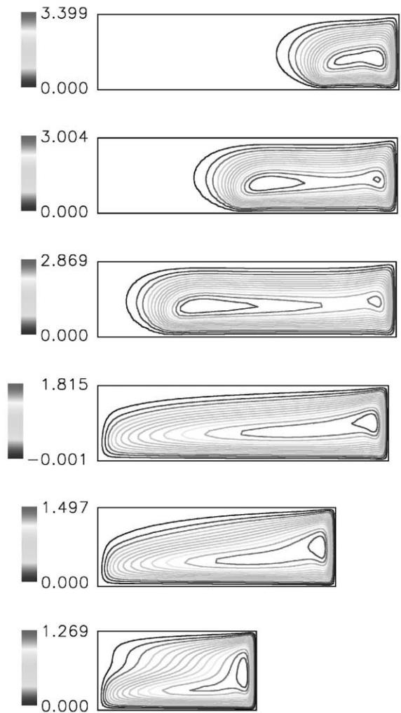
Fig. 4. Streamlines for  $Gr_s = 4.5 \times 10^5$  during solidification:  $S = 3.98, 3.96, 3.94, 3.84, 3.0$  and  $2.0$ .
