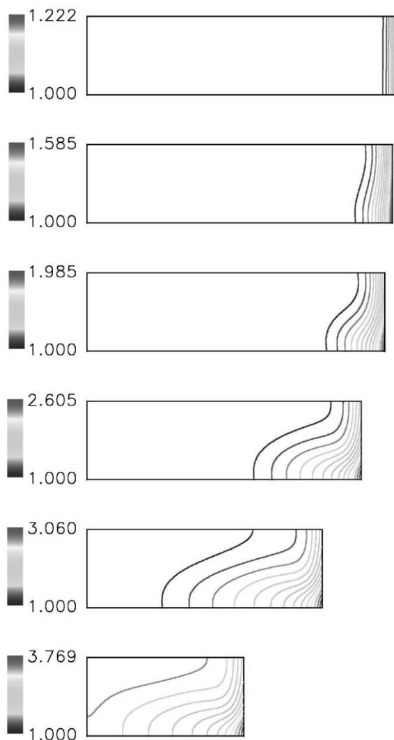
Fig. 2. Iso-concentration lines for  $\text{Gr}_s = 10^3$  during solidification:  $S = 3.98, 3.90, 3.80, 3.50, 3.0$  and  $2.0$ .
