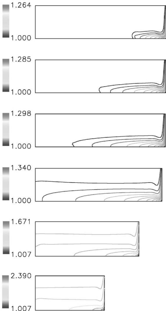
Fig. 5. Iso-concentration lines for  $Gr_s = 4.5 \times 10^5$  during solidification:  $S = 3.98, 3.96, 3.94, 3.84, 3.0$  and  $2.0$ .
