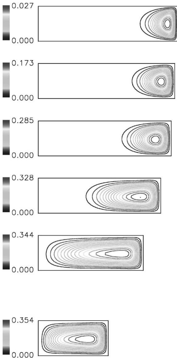
Fig. 3. Streamlines for  $Gr_s = 10^3$  during solidification:  $S = 3.98, 3.90, 3.80, 3.50, 3.0$  and  $2.0$ .
