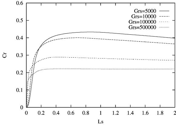
Fig. 7. Radial segregation for different  $Gr_s$ .
