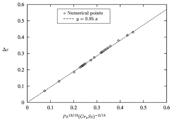
Fig. 9. Variation of  $\Delta c$  as a function of  $Pe$ ,  $Gr_s$  and  $Sc$  under the analytical model law.
