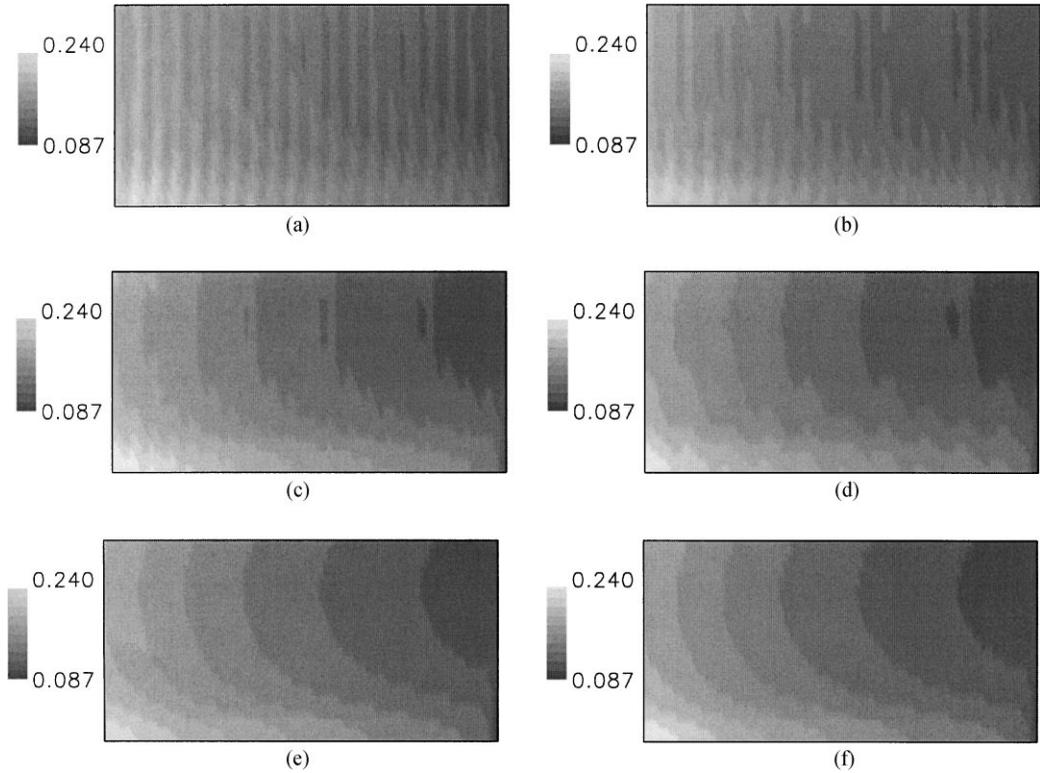
Fig. 9. Solute distribution in solidified alloy for different values of  $\alpha$  and  $T$ : (a)  $\alpha = 0.85$ ,  $T = 0.5$ , (b)  $\alpha = 0.5$ ,  $T = 0.5$ , (c)  $\alpha = 0.2$ ,  $T = 0.5$ , (d)  $\alpha = 0.2$ ,  $T = 1.0$ , (e)  $\alpha = 0.2$ ,  $T = 0.1$ , (f) non-oscillatory case.
