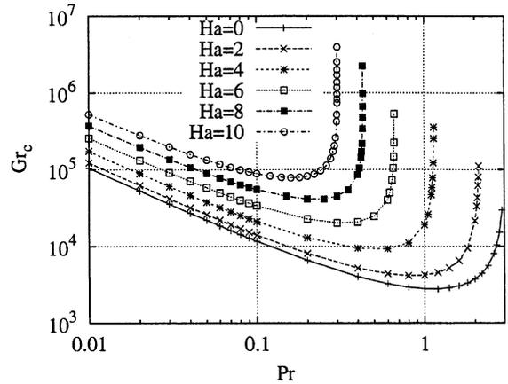
Fig. 3. Variation of  $Gr_c$  versus  $Pr$  for the oscillatory longitudinal instabilities (different values of the Hartmann number).
