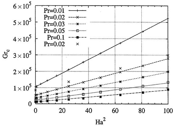
Fig. 2. Variation of  $Gr_c$  versus  $Ha^2$  for the oscillatory longitudinal instabilities (different values of the Prandtl number). The lines drawn are straight lines which approximately fit the calculated results. For  $Pr = 0.02$  are given four thresholds (indicated by X) obtained by numerical stability calculations with the method developed by Kaddeche [14].
