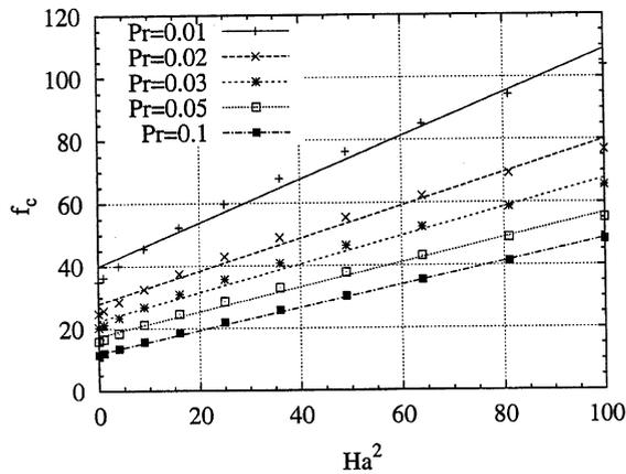
Fig. 5. Variation of the critical oscillation frequency  $f_c$  versus  $Ha^2$  for the oscillatory longitudinal instabilities (different values of the Prandtl number). The lines drawn are straight lines which approximately fit the results.
