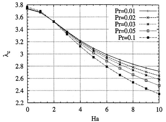
Fig. 6. Variation of the critical wavelength  $\lambda_c$  versus  $Ha$  for the oscillatory longitudinal instabilities (different values of the Prandtl number).
