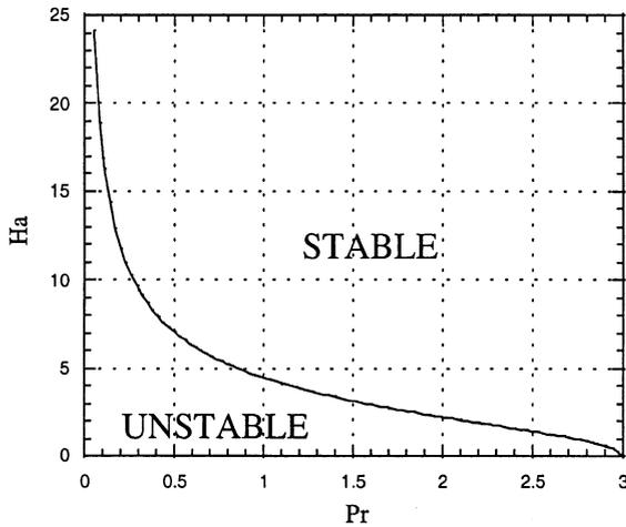
Fig. 4. Representation of the stable and potentially unstable domains (with respect to the oscillatory longitudinal instabilities) in a  $(Pr, Ha)$  plane.
